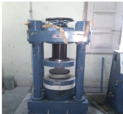
Fig 4.1 Test Set up for Compressive Strength Test
