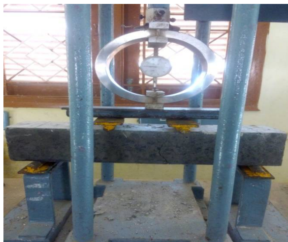
Fig 4.2 Test Set Up for Flexural Strength
